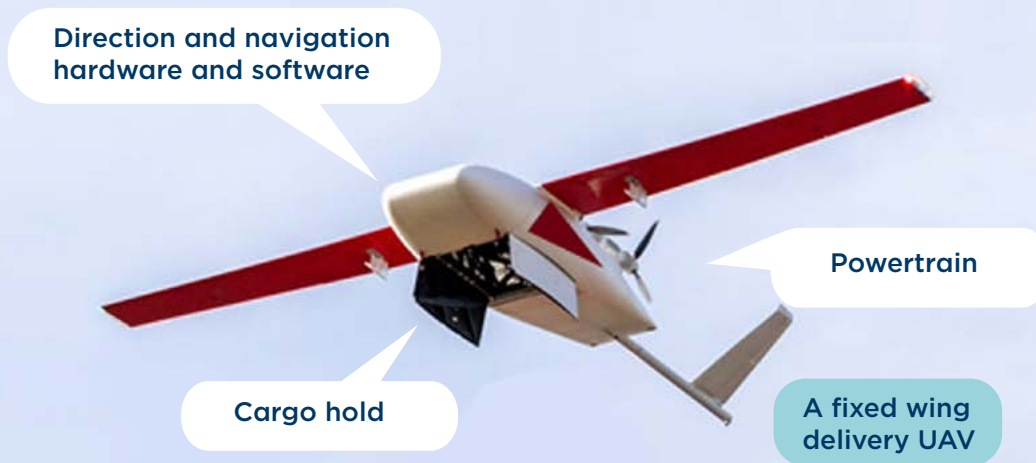
Figure 15: A typical fixed-wing delivery UAV
